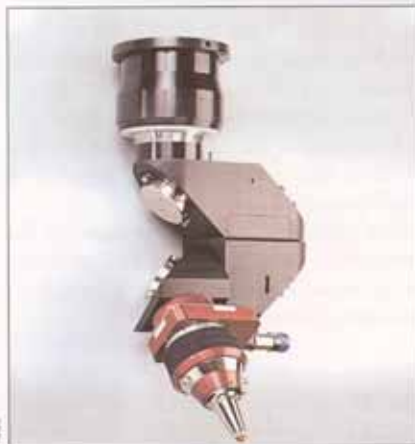
Figure 2. In-line design incorporates two motion axis with a capacitive height sensor.
