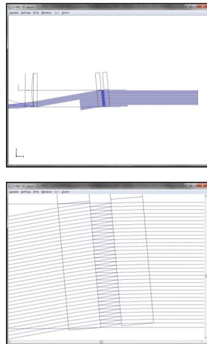
Figures 2a & 2b: BWA-CAM Optical Layout Showing Single On-Axis Ray and Zoom of the Fabry-Perot Cavity
