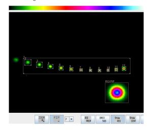
Paying attention to laser distance, placement of an iris or the use of an optical filter will help provide a more accurate and meaningful beam profile measurement of the laser's beam waist and resulting M-squared value.
