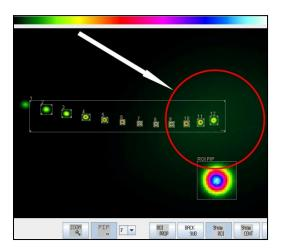
Centered about this spot and identified by the red circle, is a broad patch of light that is the light from the laser's discharge glow.
