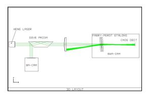
The image above shows the basic setup where the HeNe laser is very close to the measurement system. Having the laser in close proximity permits enough light to pass through to the detector and manifest as unwanted background noise.
