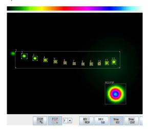
Clearly the background has been significantly reduced but not completely eliminated. One could improve this by moving the iris after the focusing lens. Another option would be to move the laser farther away from the optical setup provided the space is available.
