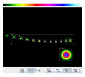
Clearly the level of background is dramatically reduced but not completely eliminated. We could move the laser further back or move the iris further forward. Another option is to insert into the BWA-CAM filter cartridge an interference filter which will
